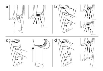
**8. Test Shade Movement** — Run the shade up and down to its limits several times, observing its movement and checking for signs of the original symptoms.
